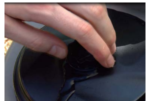
24) The air in the pump must be released ; Unscrew the air valve, release the air until he water is coming out, then screw the air valve.
