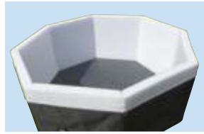
Insulating foam structure (13 cm thickness)
